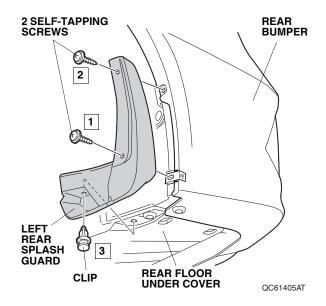
14. Turn the template over, and repeat steps 5 through13 to install the right rear splash guard on the right side of the vehicle.
